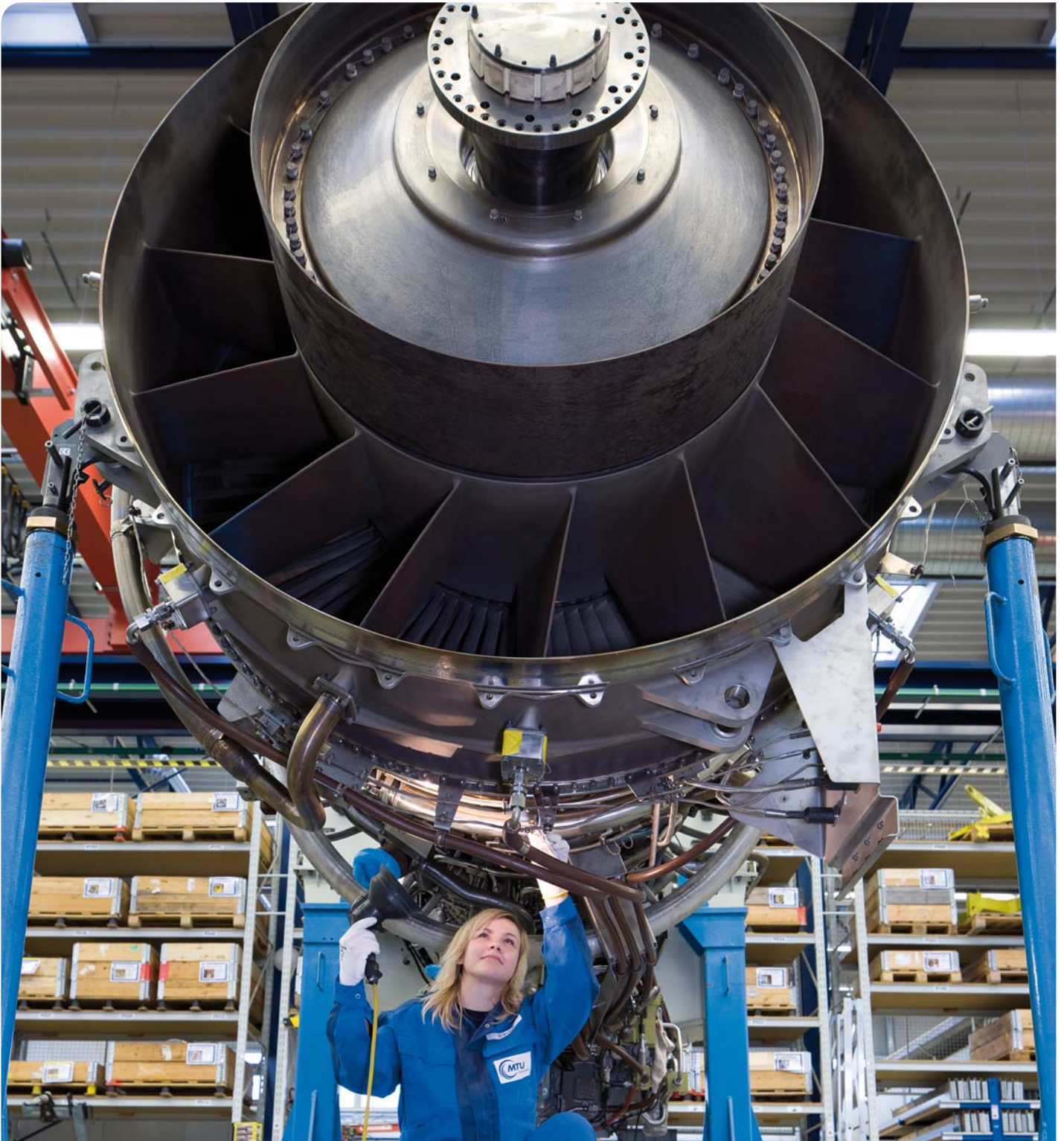
The LM6000™ is the flagship of GE's successful LM series of industrial gas turbines. It is maintained by MTU Maintenance Berlin-Brandenburg.
